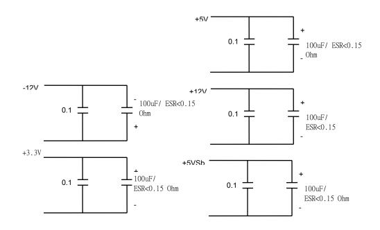
0.1uf is ceramic the other is tantalum. Noise bandwidth is from DC to 20MHz
